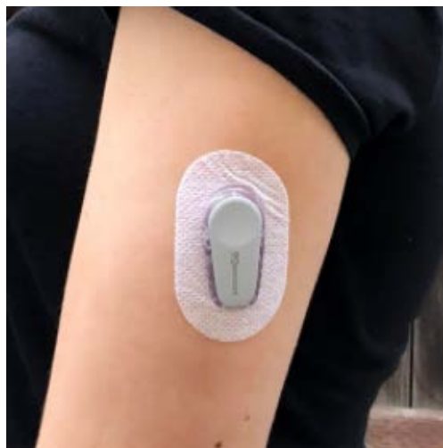
Figure 1. CGM device and related adhesive patch assembly (Dexcom G6) [6]. Photo by: Ashley Neuhaus @typelovely.
