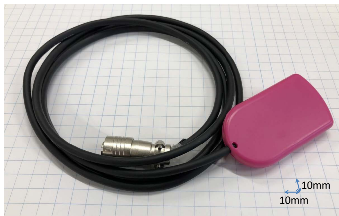
Figure 1. Prototype non-contact monitoring system for observing JVP, comprising a microwave radar sensor and patch antenna. The size of the microwave radar sensor is 45 \times 22 \times 10 mm (the housing size is 85 \times 48 \times 15 mm); transmit/receive, the carrier frequency is 24 GHz with continuous wave, and mean output power was 7 mW (maximum, 10 mW) with 10 dBi patch antenna.
