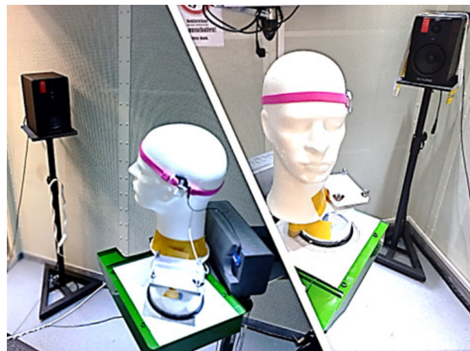
Figure 5. The figure is divided into two parts to better illustrate the measurement setup. On the left side of the ear, the speech processor is attached to the artificial head with a headband and sound is played through two loudspeakers. The axis of rotation corresponds to the axis of symmetry of the speech processor around which the head is rotated. The head shadow effects are measured via the stimulation currents.
