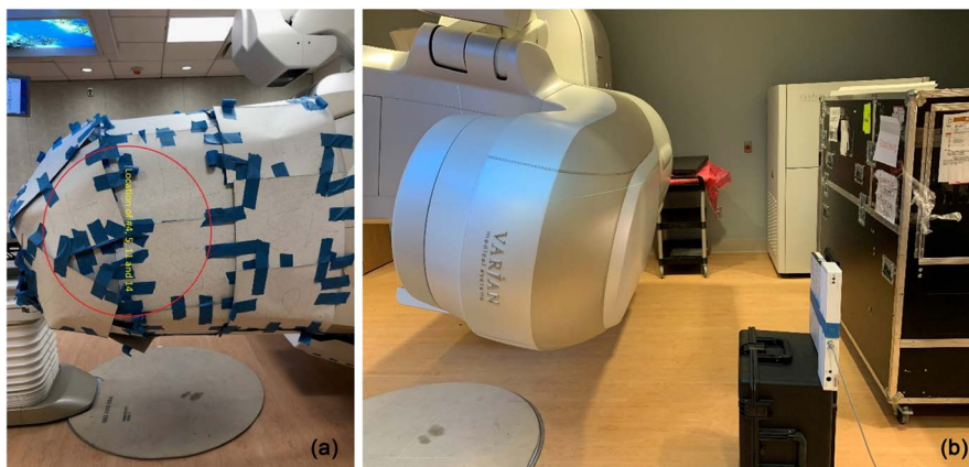
Figure 3. (a) Location of the maximum leakage from the head as determined by PPL films, and (b) measurement setup of leakage at 100 cm from the target using the IC Profiler.
