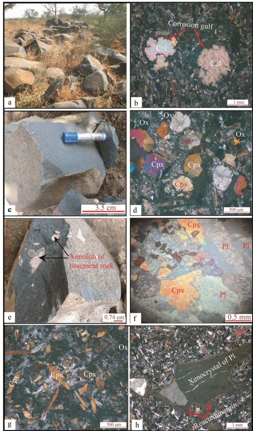
Figure 3. Aspect of some samples and microphotographs showing the structural and textural characteristics of dolerite. (a) Outcrop of a dolerite dyke in the form of bawls and blocks at Léré; (b) Microphotograph of pyrite and calcite-bearing dolerites showing calcite crystals with gulfs of corrosion; (c) Fresh sample of calcite-bearing dolerites of Léré; (d) intergranular texture with granophyre of calcite-bearing dolerites; (e) Sample of pyrite-bearing dolerites with xenoliths of basement rocks; (f) Doleritic dolerite texture of pyrite-bearing dolerites with xenoliths of basement rocks; (g) Ophitic texture of Amphibole and titanite-bearing dolerites of Poutalet (Léré); (h) Xenocrysts of plagioclase surrounded by a reactional margin in pyrite-bearing dolerites.
