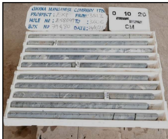
Figure 2. Loaded drill core boxes.
