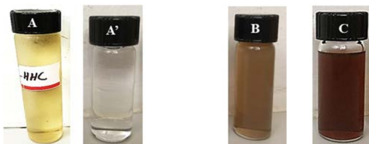
Figure 1. Daylight picture of HHC, HHC-silver salt, and HHC-AgNPs sample. A —Concentrated HH-2%, A' —HHC diluted with \text{AgNO}_3 (1 mM), B and C —HHC stabilized AgNPs sample at 15 minutes and 30 minutes of heating.
