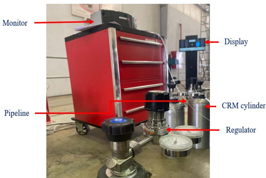
Figure 1. Calibration of CO/CO 2 monitors using CRMs.
