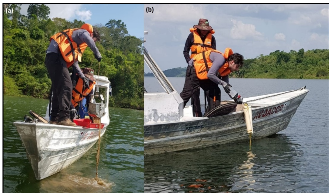
Figure 3. Dredge ready to be lowered from the boat (a) and the sediment-trap-pair deployment (b). The yield of one sediment trap quantifies silica sedimentation rate and fresh OC sedimentation rate the other.
