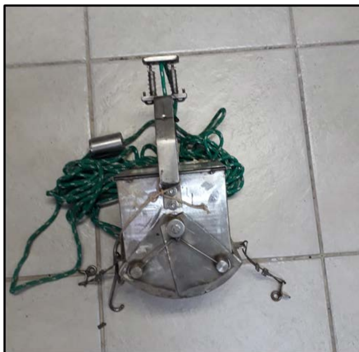
Figure 2. Ekman type dredge used for sediment sampling.
