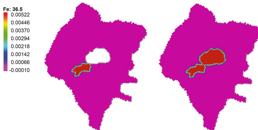
Figure 7. Transport model for layers 2 and 3 using iron at first time step of 36.5 days.
