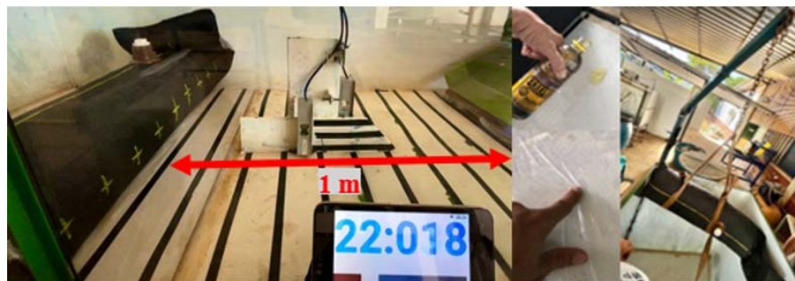
Figure 3. Flow path and equipment, barrier installed under vaseline with PVC film and crane.
