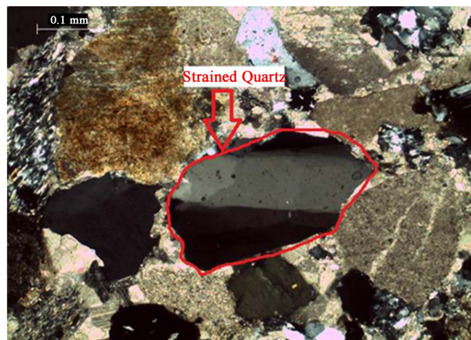
Figure 14. Photomicrograph shows strained quartz in lithic arenite of Kamlial Formation (SKM 12A), (Cross N), (I: 10 \times ).
