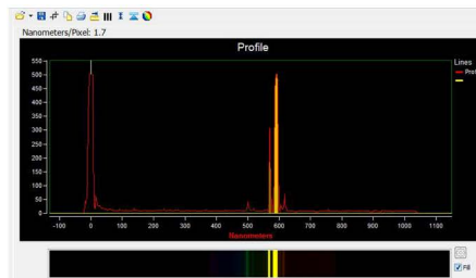
Figure 8. Sodium lamp real time spectrum.
