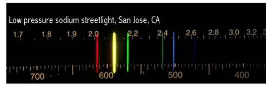
(a) Low pressure sodium streetlamp. (b) Low pressure sodium lamp spectrum wavelength.
