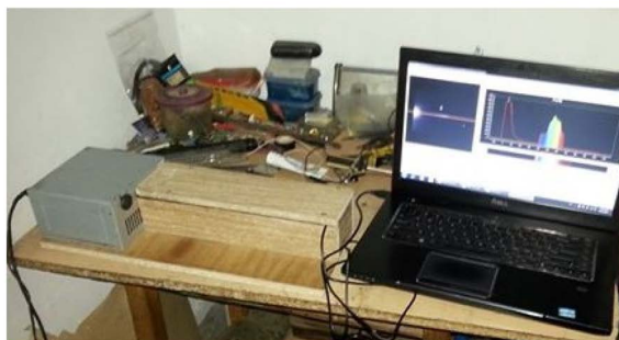
(b) Real life view of the fluorescent light Spectroscopy setup.
