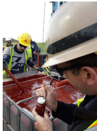
Figure 11. 18 - 24 dye test 1 m 3 -water tank being prepared with red dye.
