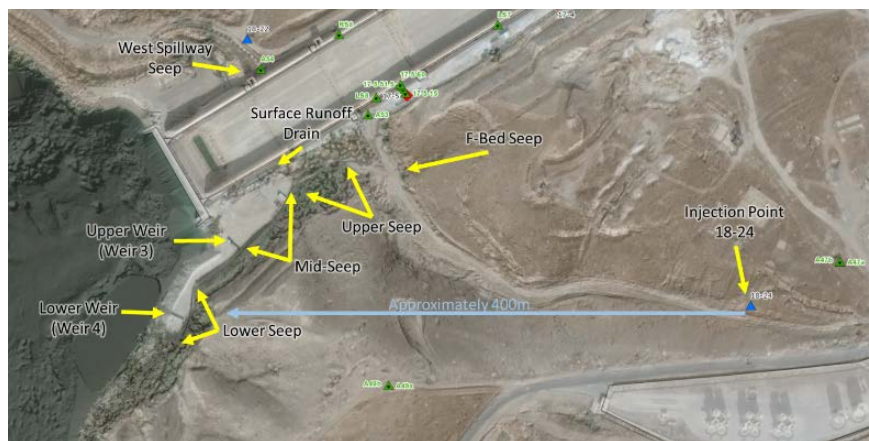
Figure 8. 18 - 24 dye test injection point and observation points.
