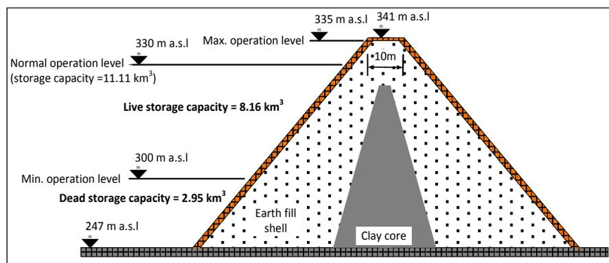
**Figure 4.** Schematic diagram of Mosul Dam cross section.
