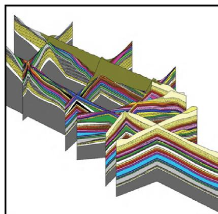
Figure 6. Intersecting cross sections from intermediate version of ERDC geologic conceptual model, showing complex stratigraphy and partial resolution of discrepancies in stratigraphy at intersections of the geologic panels from generated boreholes. (After [49]).
