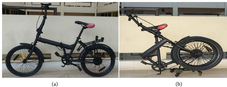
Figure 1. (a) Unfolded ( 180^\circ ) condition and (b) Folded ( 15^\circ ) condition of the product.
