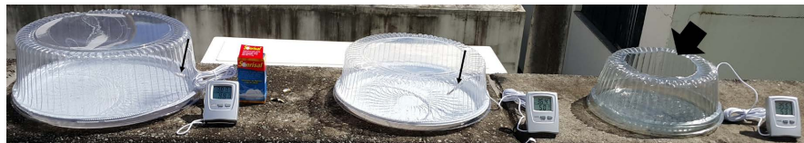
Figure 3. Similar experiments were performed in Salvador, BA (Latitude: -12^{\circ}58'16'' , Longitude: -38^{\circ}30'39'' ), using larger, round cake boxes and digital thermohygrometers with probes inserted in the boxes (thin arrows). The system allowed kinetic measurements simpler and more precise. It may be observed that the box devoid of effervescent tablet (middle) registered 36.4^{\circ}\text{C} ( 97.5^{\circ}\text{F} ), whereas the box that received the tablet (left) displayed 38.7^{\circ}\text{C} ( 101.6^{\circ}\text{F} ). Another box with removed cover top (thick arrow), as a control (right), presented 35.5^{\circ}\text{C} ( 95.9^{\circ}\text{F} ).
