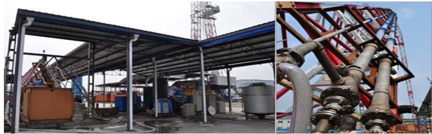
Figure 3. “Virtual and real combination” simulation experiment bench with large multi-phase flow at any angle and 36 meters in height.
