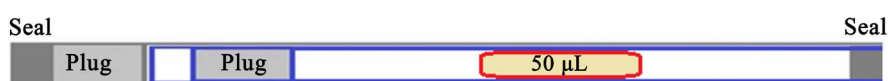
Figure 1. The straw-in-straw system loaded with 50 µL sperm and heat-sealed at both ends. The straw-in-straw system was made by inserting a 0.25 mL straw loaded with sperm into a 0.5 mL straw with their plug ends placed on the same side.
