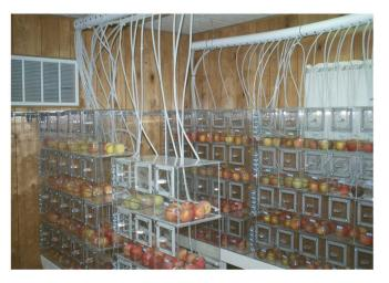
**Figure 1.** Ripening chambers at the University of Idaho Pomology and Viticulture Program laboratories were used to evaluate evolved ethylene and respiration of apples.
