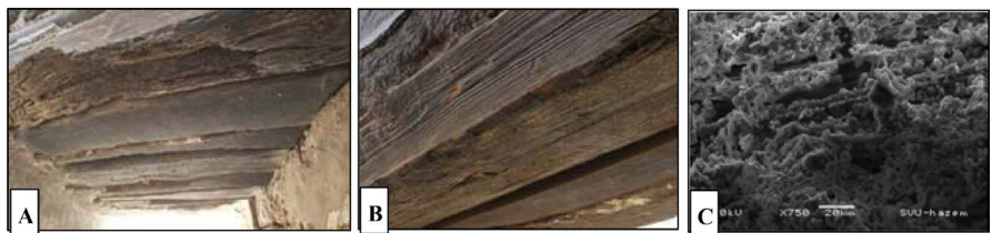
Figure 2. (A)-(C), shows the burn of some window lintels in the outer portico of Fatma Khatun mausoleum, (C) SEM micrograph. 20 \mu m.
