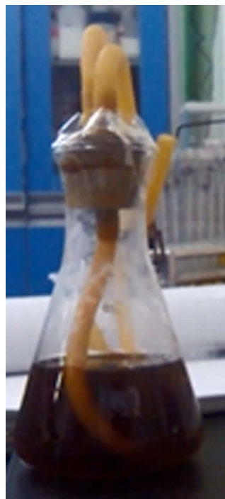
Figure 1. The fermenter for biohydrogen production.
