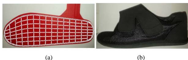
Figure 1. (a) Pedar-X System wide insole with superimposition of sensor map; (b) Smoothed semirigid Terapes shoe used to collect reference data.
