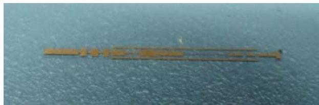
Figure 8. MIC card of mixer on 2 mil quartz substrate.
