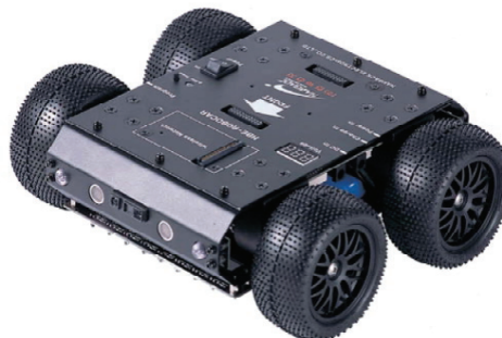
(a) One experimental car with PSD sensors and ultrasonic sensors.
