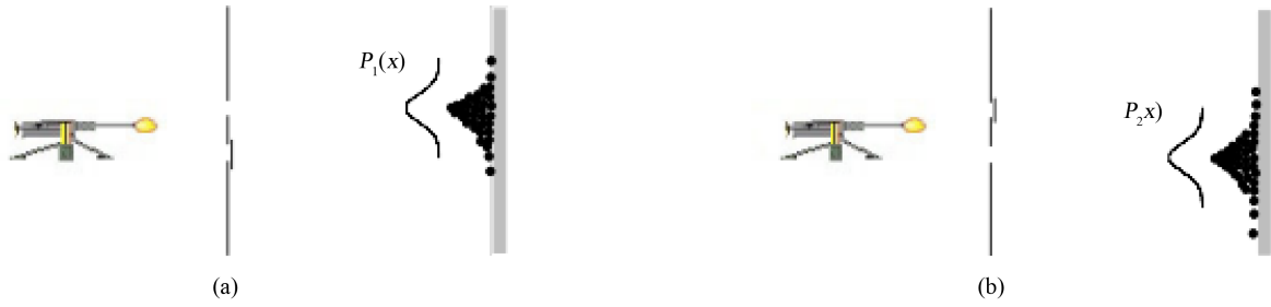
Figure 1. Edge-on view of particle source, two-slit diaphragm, and detection screen with respective patterns for situation A (top-slit open; bottom-slit closed) and situation B (top-slit closed; bottom-slit open).
