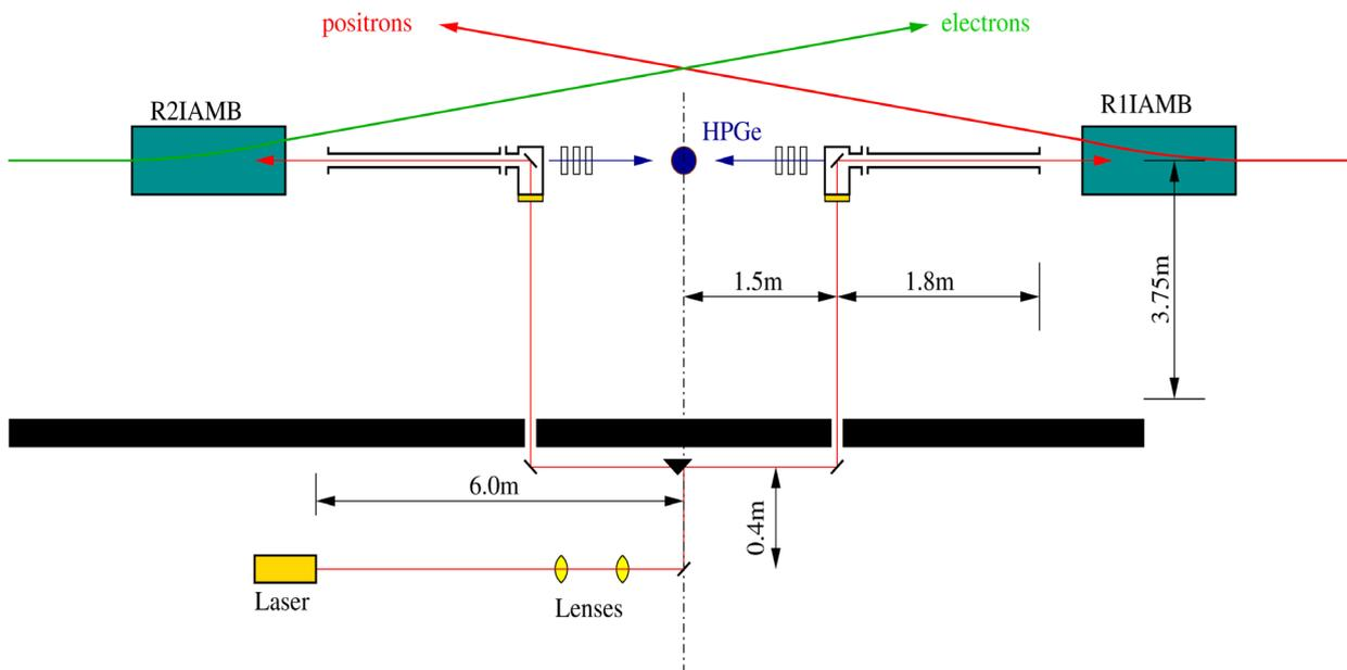
**Figure 2.** Simplified schematic of beam energy measurement system. The positron and electron beams are indicated. R1IAMB and R2IAMB are accelerator magnets, and the HPGe detector is represented by the dot at the center. The shielding wall of the beam tunnel is shown cross-hatched, and the laser is located outside the tunnel.
