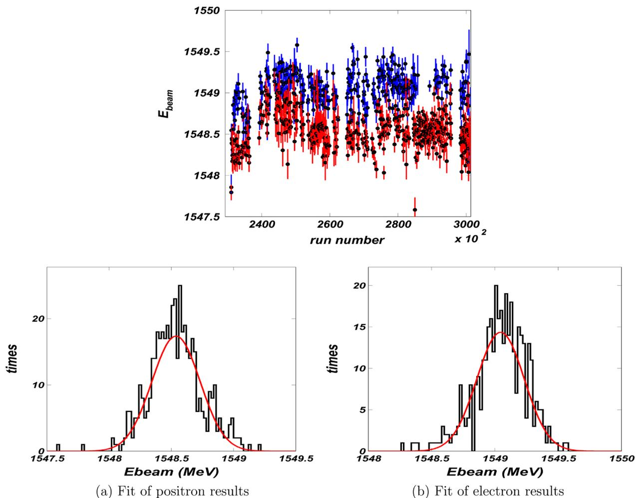
**Figure 1.** Beam energy measurement results during the  $J/\psi$  data taking. The horizontal coordinate is the running number; the points with blue error bar are results for electron beam, while the points with red error bar are for positron beam. The averaged energy values for electron and positron beams are respectively  $1549.0 \pm 0.2$  MeV and  $1548.5 \pm 0.2$  MeV, with corresponding deviations of  $0.20 \pm 0.01$  and  $0.19 \pm 0.01$  MeV.
