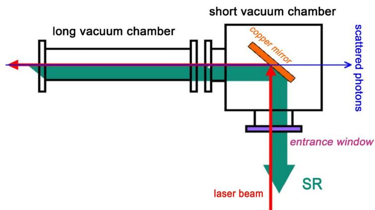
**Figure 5.** Schematic diagram of the laser to vacuum insertion of BEMS. SR represents the Synchrotron Radiation light.
