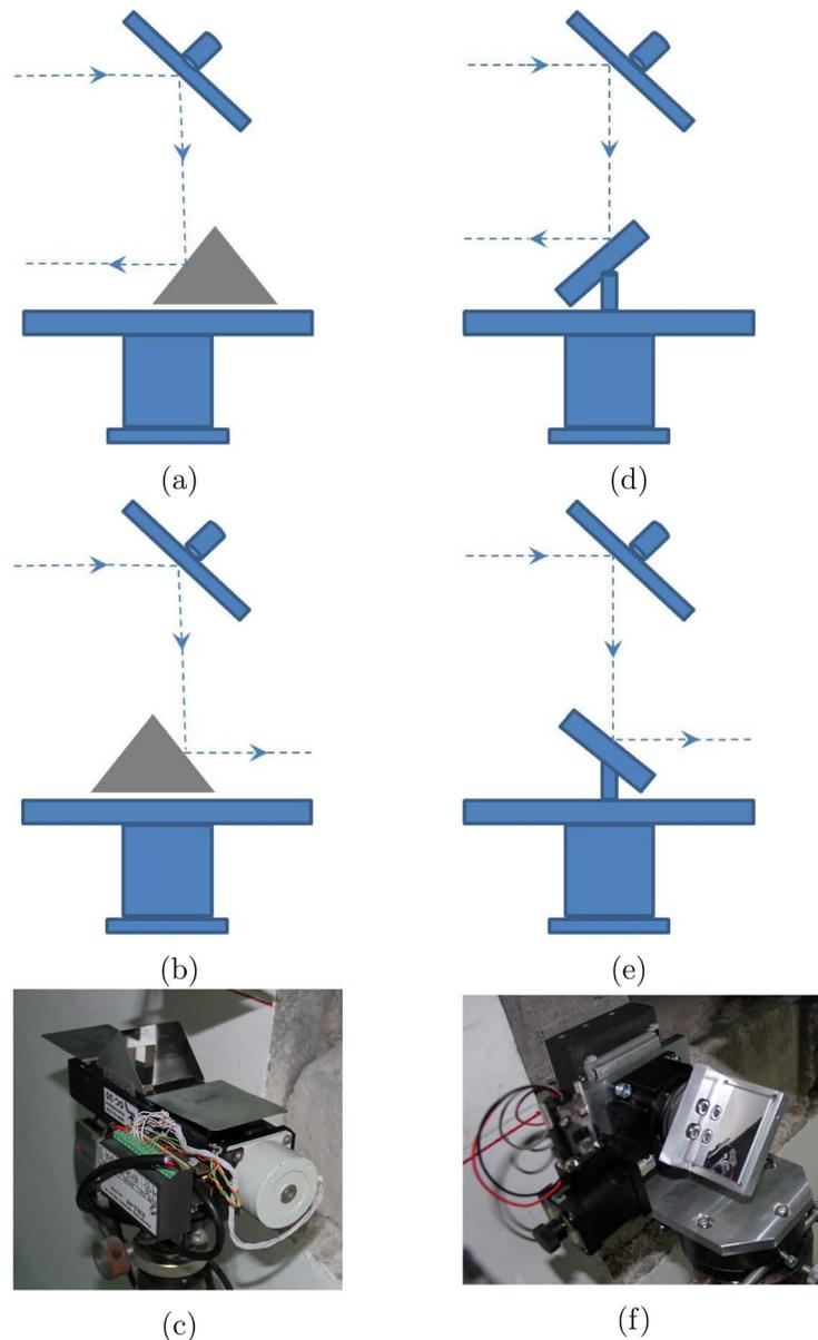
**Figure 3.** The left side is the translatory prism and the right side is the rotary platform. The laser light, represented by the dash line, is reflected to the electron ((a), (d)) and positron ((b), (e)) side using translatory prism and rotary platform respectively. The assembly pictures of translatory prism and rotary platform are shown in (c) and (f) separately.
