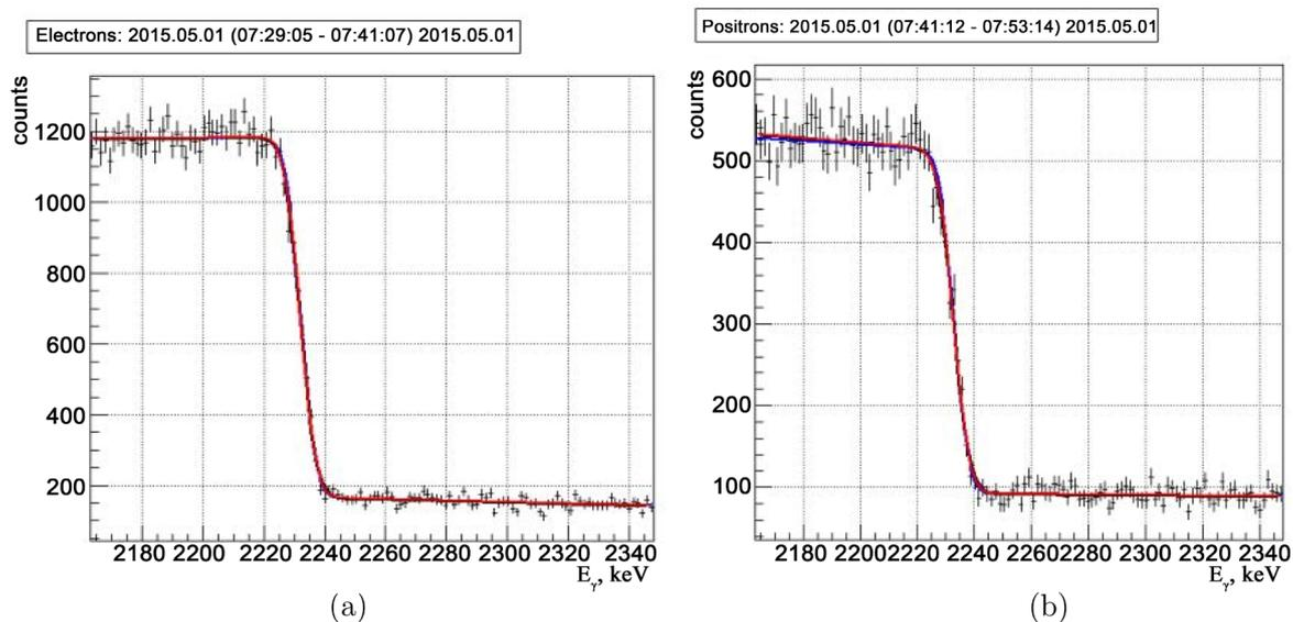
**Figure 11.** The measured edge of the scattering photons energy spectrum. The line is the fit result. (a) Electron case, (b) Positron case.
