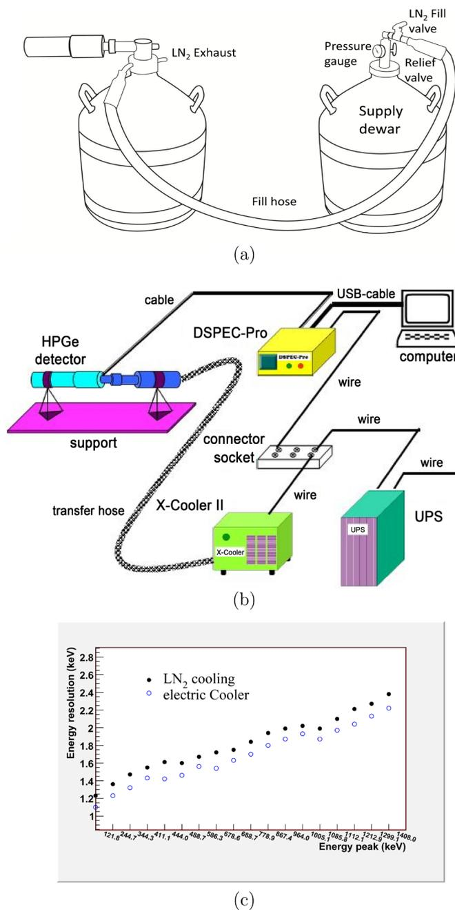
**Figure 7.** The HPGe detector cooled by two different refrigeration modes and the corresponding performance. (a) The LN<sub>2</sub> cooling case, the LN<sub>2</sub> is transfer using the self-pressuring system. (b) The electric cooler case. (c) The comparison of the detector resolutions to the characteristic lines of <sup>152</sup>Eu under LN<sub>2</sub> cooling method represent as dot and electric cooler case indicated as circle.
