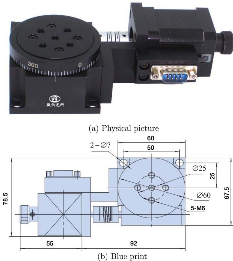
**Figure 4.** The rotary platform stage adopted by BEMS. (a) shows the physical picture of the rotary platform, which is connected with the step controller by RS232 cable. (b) shows the blue print of the rotary platform where the detailed dimensions are presented.
