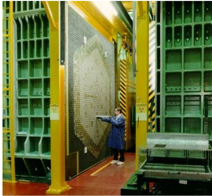
Figure 1. Experimenter loading fuel in the ZPPR reactor.
