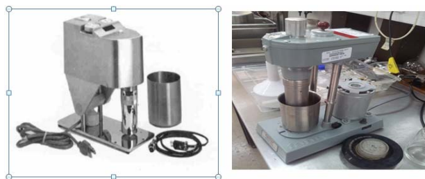
Figure 5. Viscosity measuring instrument.
