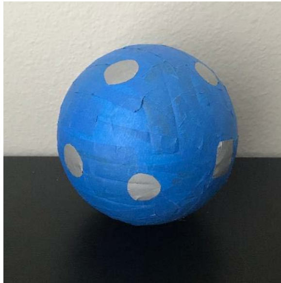
Figure 4. Ball and its reflective markers.
