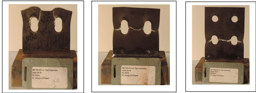
Figure 5. Failure modes of shear tab specimens under tensile load.
