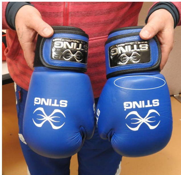
Figure 24. Deformation near wrist region of Std 10 oz glove after 253 drops on to a force plate. The area of deformation is indicated by the white ellipse. A glove with which the dropped glove formed a pair is shown for comparison.
