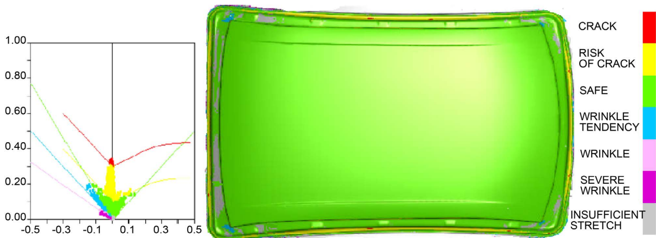
Figure 9. Forming limited diagram—FLD (Modified tooling of forming simulation result).
