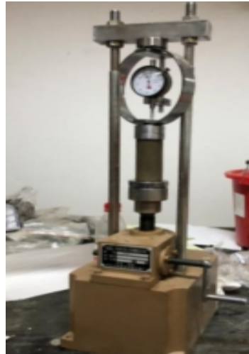
Figure 3. YYW-1 manual lime soil unconfined pressure gauge.
