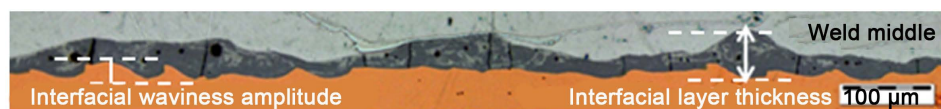
Figure 8. Detail of the interfacial layer morphology in the weld middle and indication of the interfacial waviness amplitude and interfacial layer thickness.
