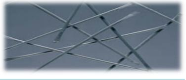
Figure 1. Steel fibers.
