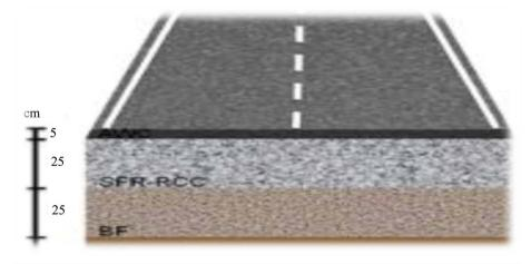
Figure 7. Composite pavement with steel fiber or SFRC.
