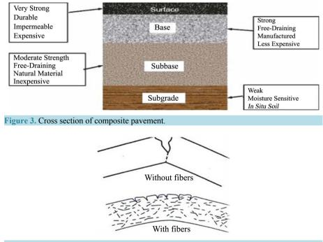
Figure 4. Failure mechanism of pavement and the "effect of fibers".
