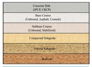
Figure 2. A typical cross-section of a rigid pavement layers.
