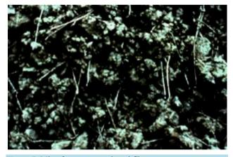
Figure 8. Mix of aggregate and steel fiber.
