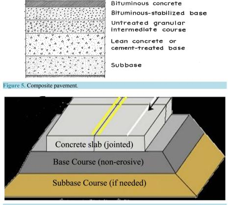
Figure 6. Rigid pavement like structure.
