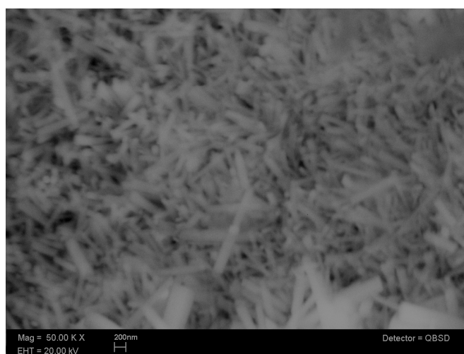
Figure 4. SEM Image of the particles obtained at 120°C without the action of the CTAOH.
