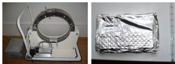
Figure 4. (a) Configuration of experimental device with applicator and pulse generator for the SHIELDED version of the experiment. Mounted on the bottom inner part of a pair of toroidal coils is the 96-wells titration plate A in an earthed cover with 48 wells containing the suspension of bacteria E. coli ; (b) Detail of plate B wrapped in a similar earthed cover with 48 wells filled with bacterial suspension.
