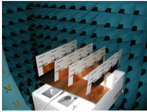
Figure 19. 4x4 array with non equilibrate power repartition in the near-field anechoic chamber.
