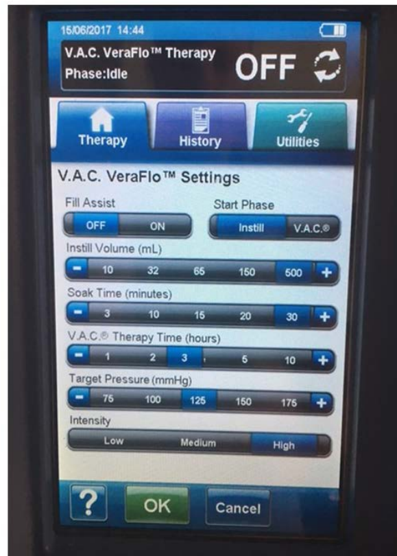
Figure 2. V.A.C. Veraflo™ Therapy settings for the intraabdominal irrigation of Vashe® (500 cc's over 30 minutes every three hours) alternating with continuous suction at 125 mmHg.
