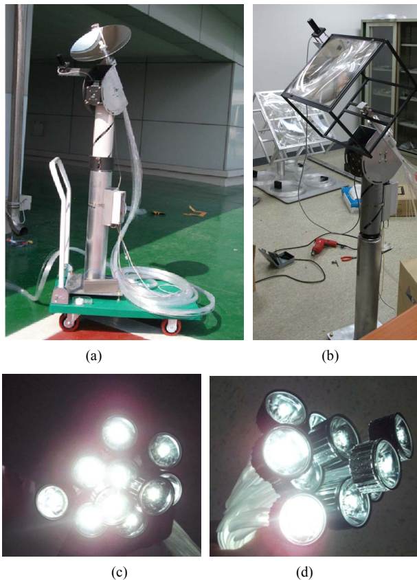
Figure 4. Hardware schematic using (a) reflectors and (b) lenses. Experimental results showing (c) uniform illumination and (d) non-uniform illumination.
