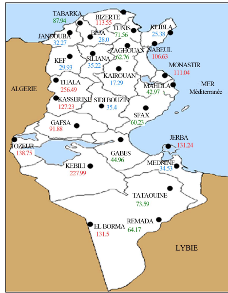
Figure 4. Available power density from wind at 11 m height in an open area (in W/m 2 ).
