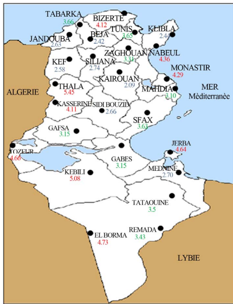
Figure 3. Annual mean wind speed at 11 m height in an open area (in m/s).
