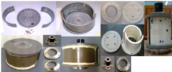
Figure 3. Pictures of two split reaction water turbines.
