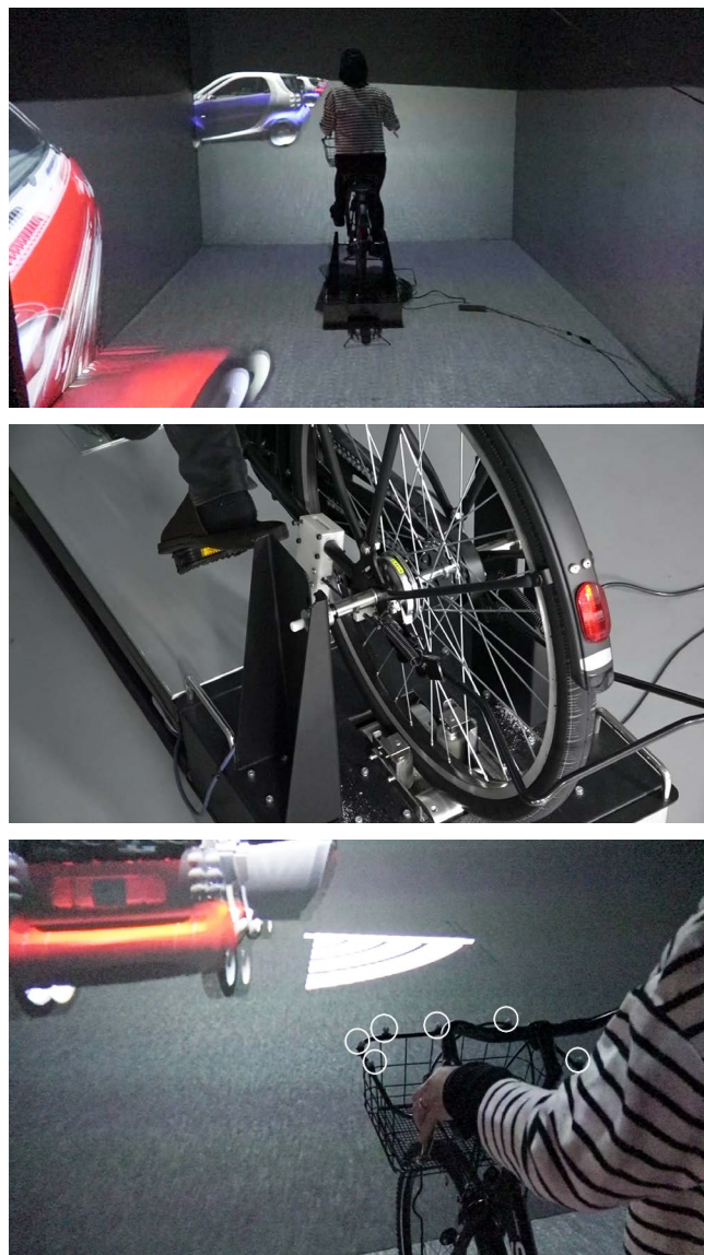
Figure 1. (Top) The cycleStreet system installed in the CAVE. (Middle) The cycleStreet roller for detecting the rotation speed of the back wheel. (Bottom) The markers (highlighted by circles) for measuring the bicycle's direction of movement.
