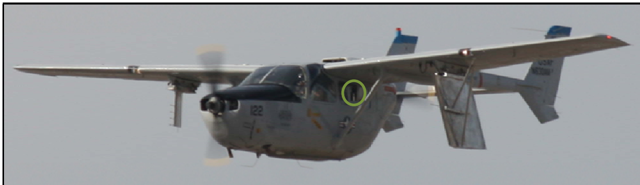
Figure 1. Cessna O-2A Skymaster with SWIFTER on the port outboard hardpoint with the IR camera port circled in green.
