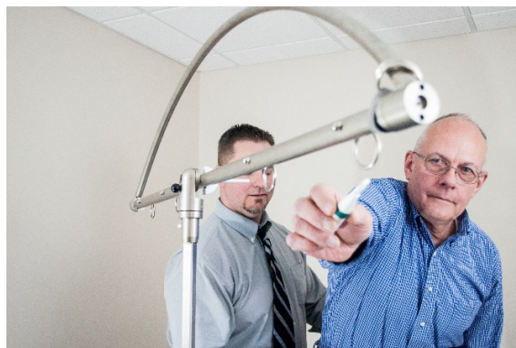
Figure 1. The dynamic arc. Image of patient reaching to place a marker on a hook of the balance arc.
