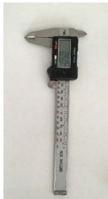
Figure 1. Thickness measurement of specimens by a digital caliper.
