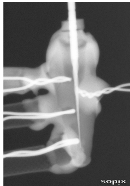
Figure 1. Each test specimen was constructed by placing three thermocouples inside the root canal; in addition, one thermocouple was attached to the surface of the root canal.
