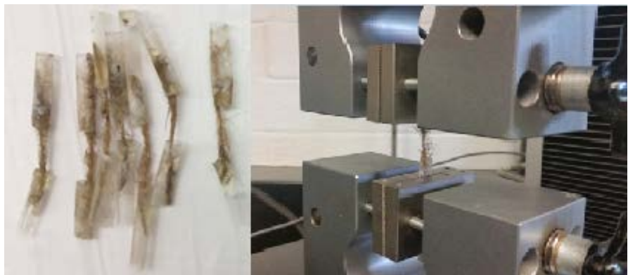
Figure 4. Testing of samples covered with epoxy at the end (Method-II).
