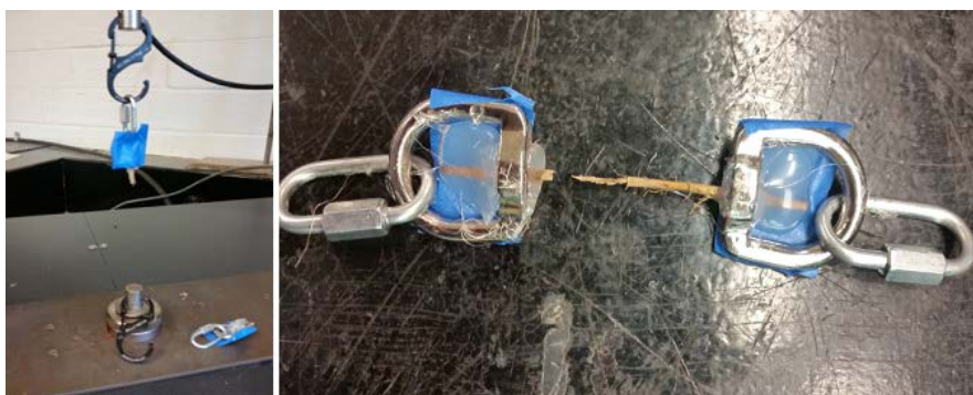
Figure 6. Ruptured sample after the tensile testing using Method-IV (left) and Method-IVEx (right).
