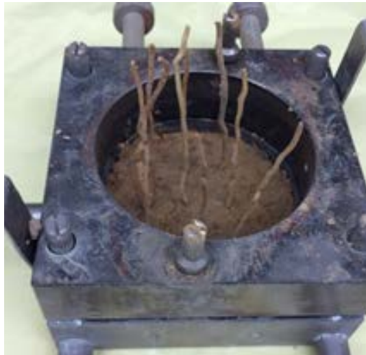
Figure 12. Manually planted root sample inside the shear box of direct shear test machine (after [27]).
