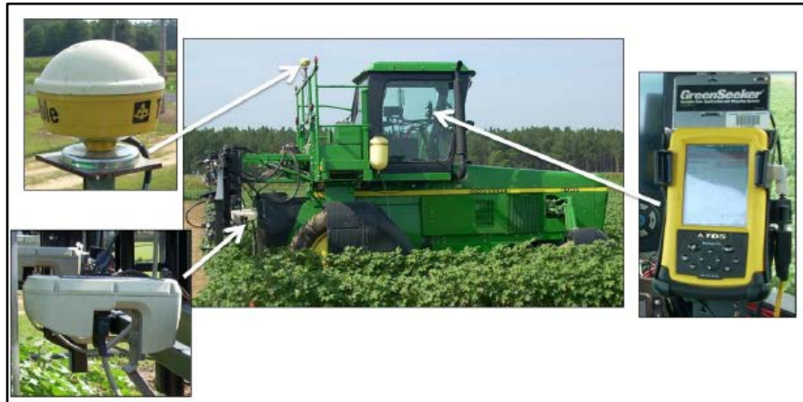
Figure 2. The sprayer-mounted GreenSeeker ® RT-200 system.
